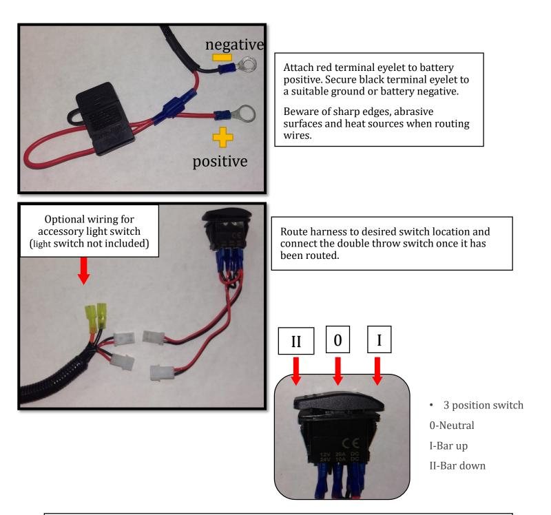
Switch may be left in position I or II, which will keep indicator LED on. In order to turn off indicator LED, move switch to neutral position.
