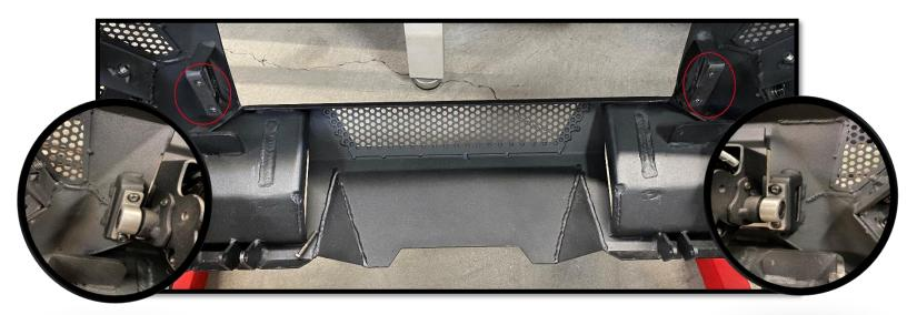
• Remove the preinstalled static light bar mount from the Element bumper. You'll need to reuse the hardware to mount the power light bar mount. Use ¼" x ¾" Button head bolt to secure the power bar to the backside of the Element bumper. Each side will use two screws. Refer to the image above (red circles).
