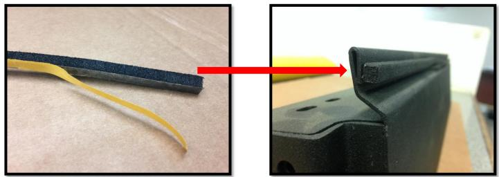
• Install the ¼"x 21" foam strip on the power bar bracket front side. Refer to the image above. Be sure the surface is clean. Prepare the inside surface of the bracket where the foam strip will be mounted with Isopropyl alcohol. A clean, dry surface is required in order for tape to stick properly. If needed, apply 1 glue drop in the glue tape, and apply pressure for about 10 - 15 seconds for better adhesion.
