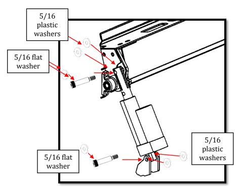
• Periodically inspect hardware and tighten as needed. If you need the actuator rod to extend further out or retract it in, you can manually do so my turning the rod clockwise to extend it or counter clockwise to retract it.
