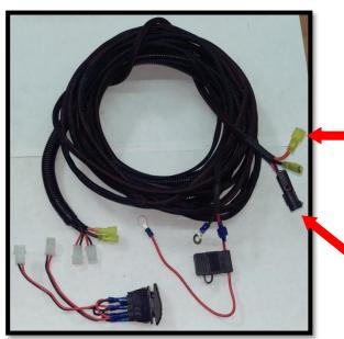
With the actuator installed, connect the female plug to the male plug of the actuator. Run the power/ground leads to the battery. Be sure to connect the positive side to the positive terminal of your battery and the negative side to the negative terminal of your battery. The excess wire can be secured with electrical tape or zip ties. Please reference to the light bar manufactures manual on how to wire it up.
