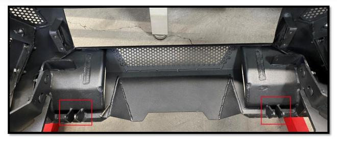
• Due to the symmetrical design, you can mount the actuator on the left or right side of the bumper. You will need to pick a side before you begin installing the actuator. Referenced in the image below (red squares)
